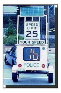
This is a mobile trailer-mounted radar display that measures each approaching vehicle's speed and displays it next to the legal speed limit in clear view of the driver. This element is applicable on any street where speeding is a problem and can be moved from location to location easily.
