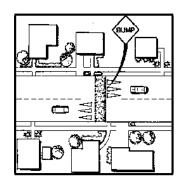
Speed humps are rounded raised areas placed across the roadway. They are generally 10 to 14 feet long (in the direction of travel), making them distinct from the shorter "speed bumps" found in many parking lots, and are 3 to 4 inches high. The profile of a speed hump can be circular, parabolic, or sinusoidal. They are often tapered as they reach the curb on each end to allow unimpeded drainage.
