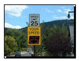
Speed feedback signs perform the same functions as radar trailers but are permanent. Real-time speeds are relayed to drivers and flash when speeds exceed the limit. Speed feedback signs are typically mounted on or near speed limit signs and can be mobile units.
