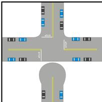
Full street closures are barriers placed across street to completely close the street to through-traffic, usually leaving only sidewalks open.
