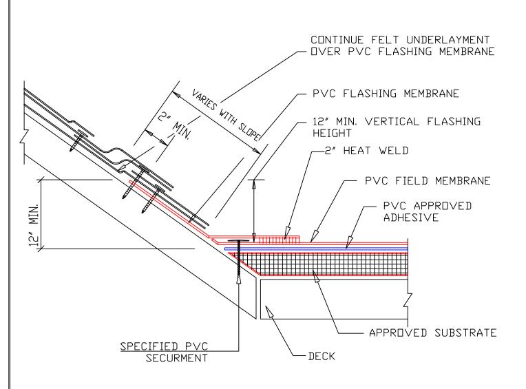
NOTE: THIRD COURSE OF SHINGLES MUST OVERLAP FLASHING MEMBRANE
