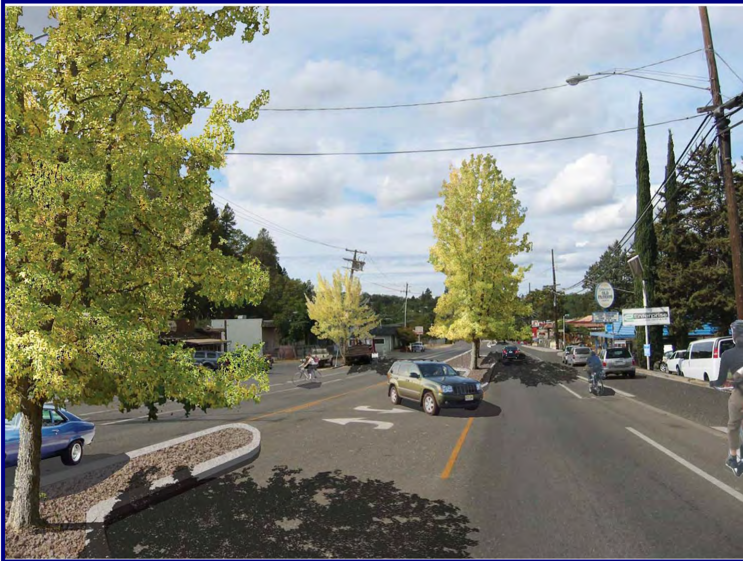
Exhibit 5-6: Visualization with 2 Lanes Plus Parking (Convertible to 4 lanes without parking if necessary)
