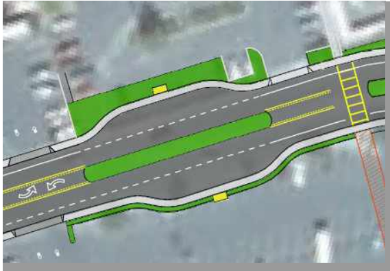
Figure 11: Conceptual roadway design with transit pull out
