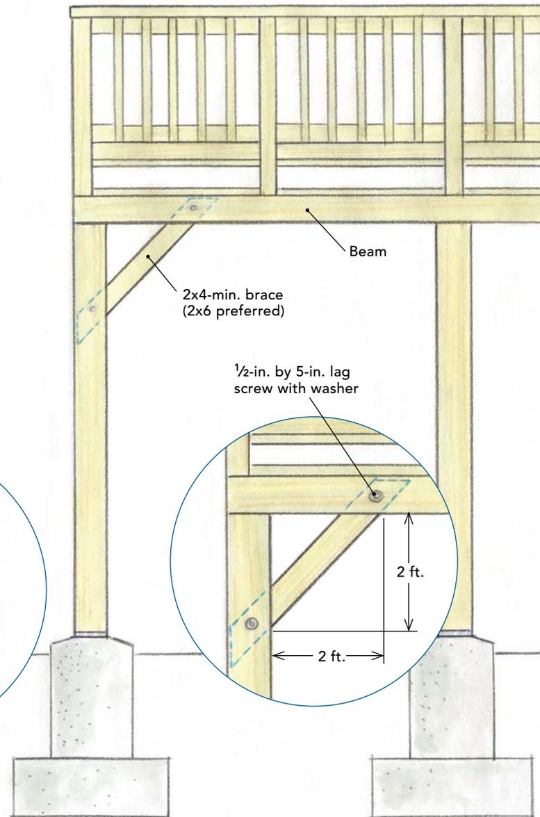
**THE FIX** **Brace and fasten the posts**
